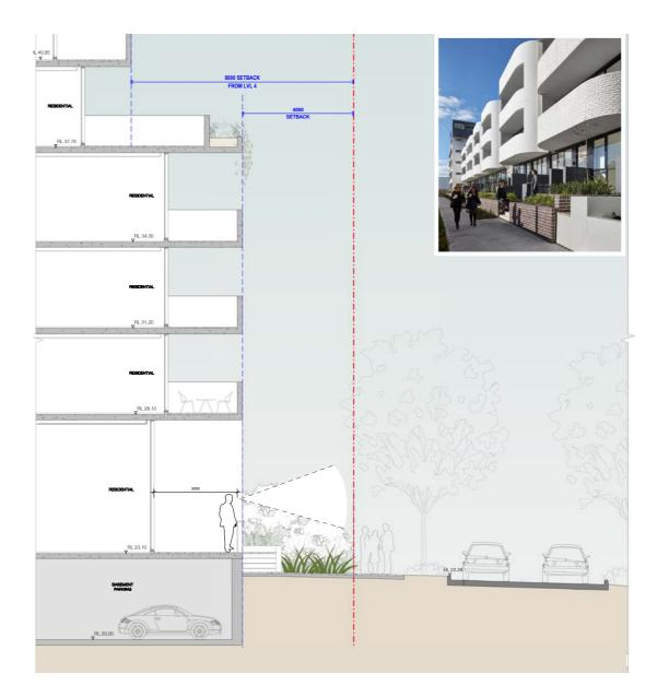
All ground floor residential apartments are to be raised above street scape level to provide passive surveillance to public domain and to create visual privacy within each apartment. Sight lines will be enabled by transparency at ground level
