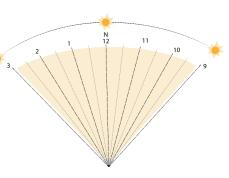
The diagram to the right shows how a typical floor plate achieves the solar access requirements of the ADG on the winter solstice
